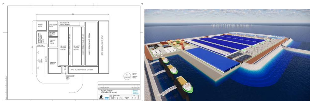
Figure 10 a) A typical energy island plot plan. This specific plot plan is for Scenario 2b - 5 GW 30% hydrogen conversion. b) a 3D impression of the 5GW-70% hydrogen conversion scenario.
