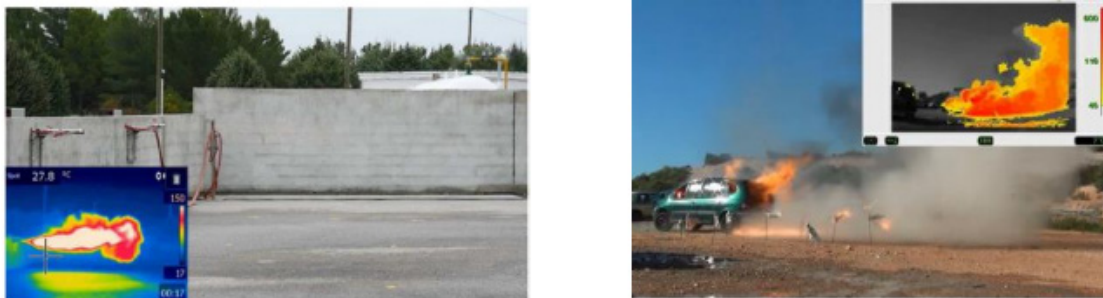
Figure 1 - Hydrogen fire [4]: Left picture – Ignited hydrogen only visible with a thermal camera, thermal radiation falls off sharply around the flame. Right picture – Experiment with a hydrogen vehicle fire. Flare at the hydrogen vehicle (700 bar), visible part of the flame is small most of the flame is invisible.
