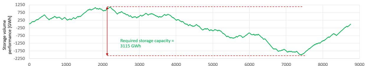
Figure 4.44: Annual storage volume profile. Positive values represent injection, while negative values indicate withdrawal. The total required storage capacity is 3.11 TWh.
