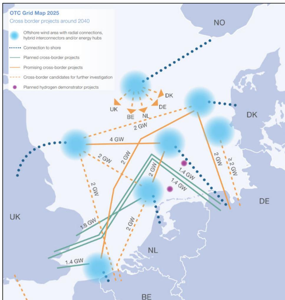
Figure 2.14: OTC electricity grid map 2025, displaying planned and promising cross-border (interconnector) projects until 2040 (source: [OTC expert paper III](#)).
