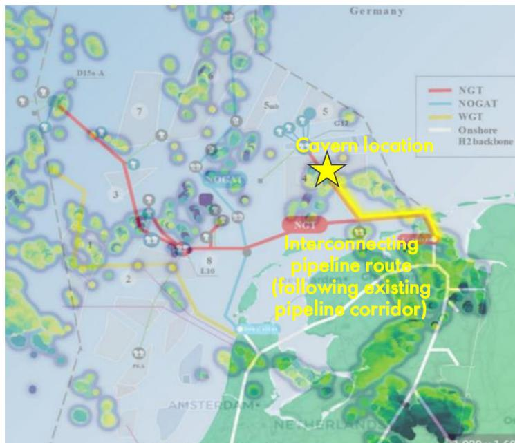
Figure 4.50: Location of offshore salt cavern in the M2 block (near the G17 block) for the case study conducted by Shell and Gasunie.
