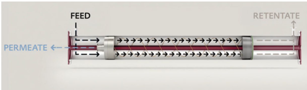
Figure 14 – Schematic principle of membrane separation.
