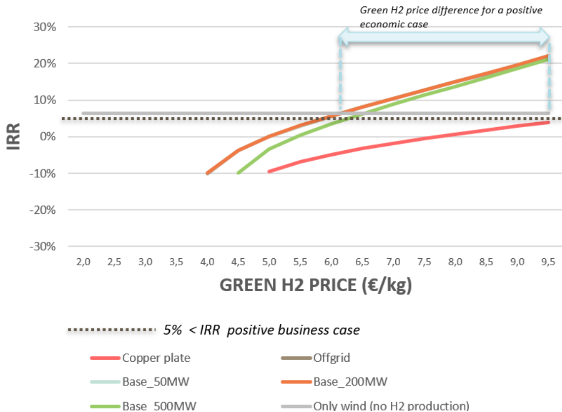
Figure 5 Economic feasibility of the different grid configurations for the DEMO 2. Assumptions: no grid tariffs included to pay when consuming electricity, no infrastructure costs for H2 and electricity, no subsidies or premiums for wind and H2, no start-up or ramp-down costs of electrolyzers. CAPEX offshore electrolyzers is assumed for this calculation on 4000€/KW.
