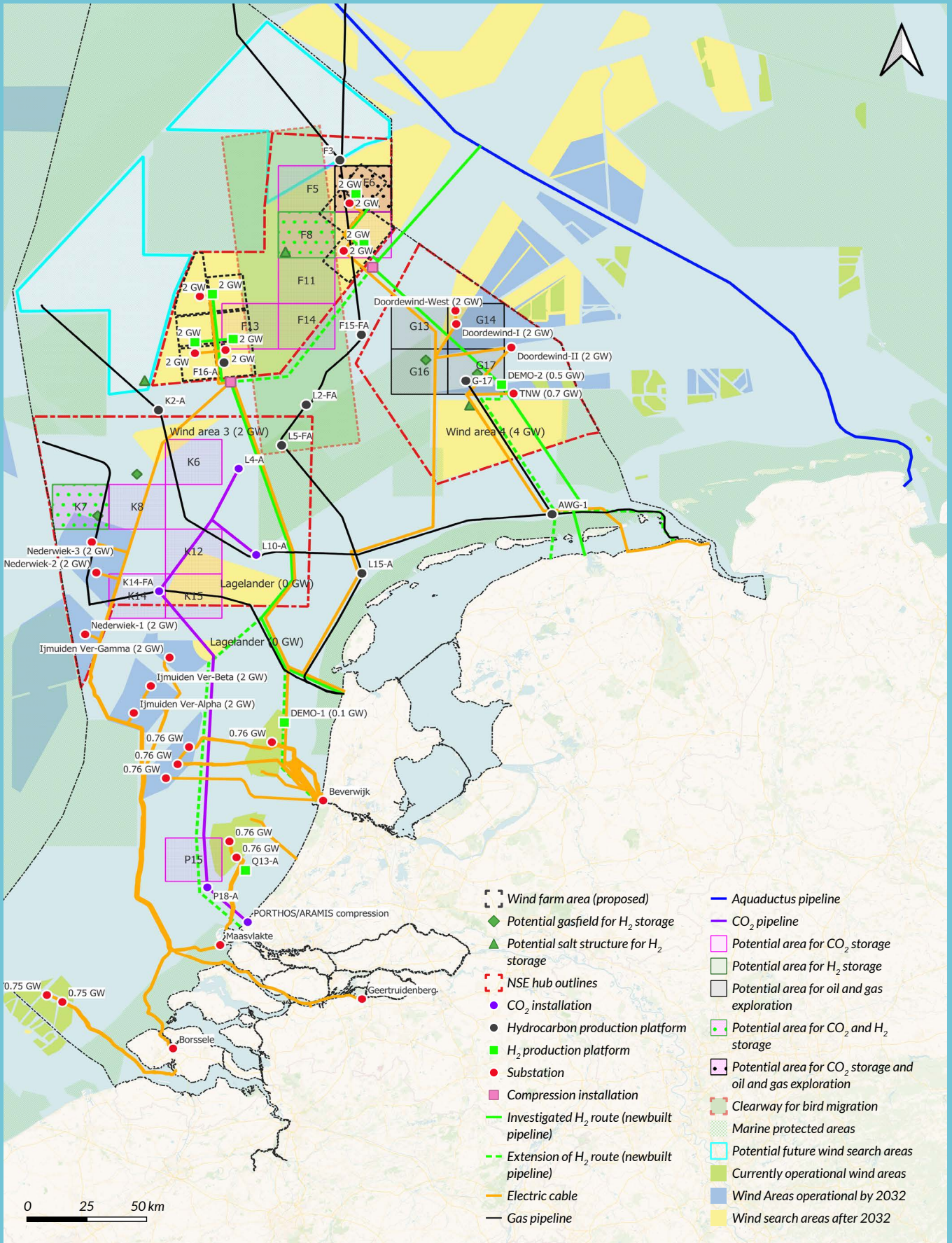
Figure 2: Vision of the North Sea in 2050 with blueprints of the three NSE hubs according to the ambitious NSE5-NAT scenario with 70 GW offshore wind and 20 GW offshore hydrogen production, and transport infrastructure of electricity and hydrogen (all new built in this particular scenario).
